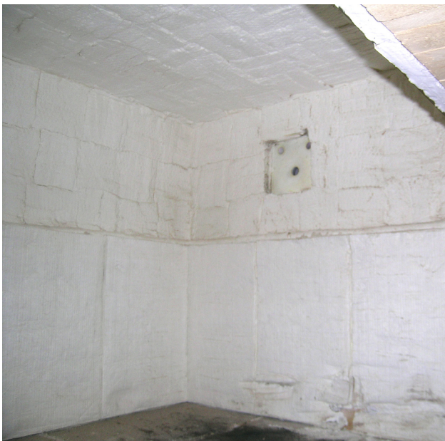
Views showing burner mounting locations at opposite ends. Burners are staggered to increase circulation and temperature uniformity
