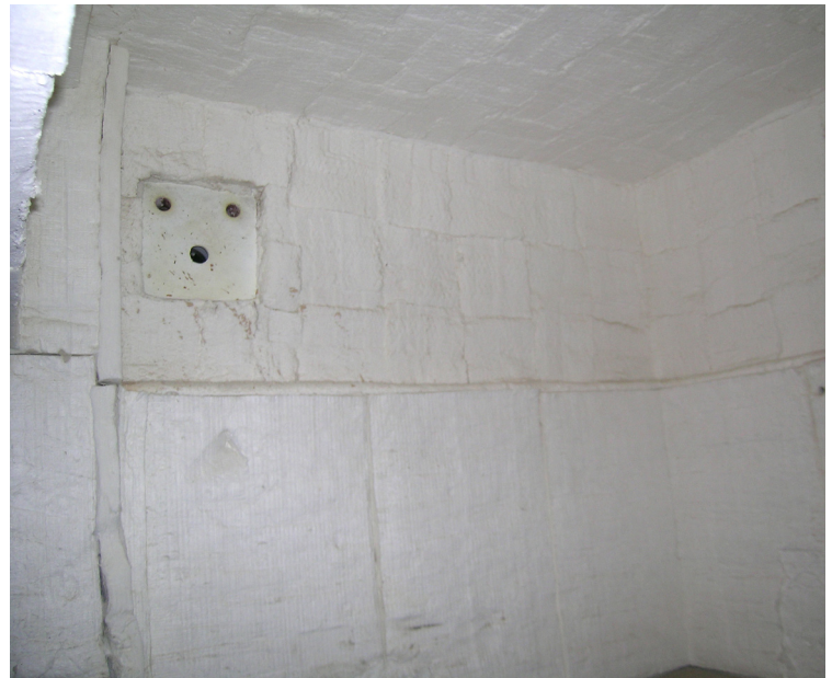
Views showing burner mounting locations at opposite ends. Burners are staggered to increase circulation and temperature uniformity
