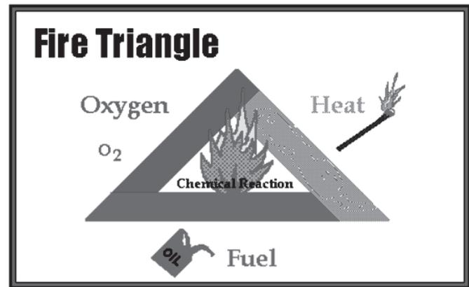
**Figure 2.1 Oxygen Fire Triangle**
