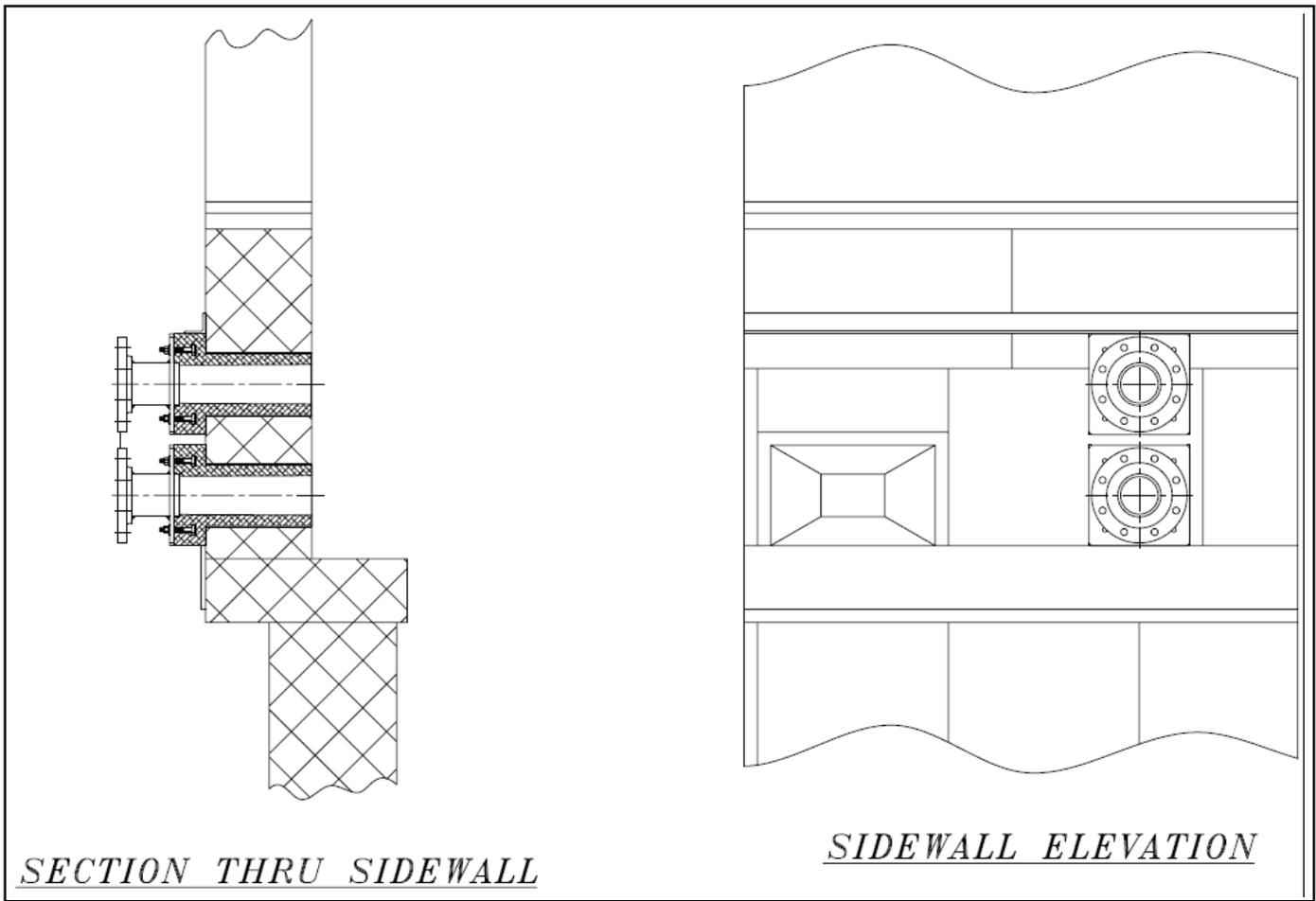
Figure 3.9. SideWall Injector Layout - Endport Furnace
