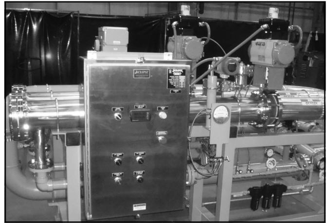
**Figure 4.2. Air Flow Control Train**
