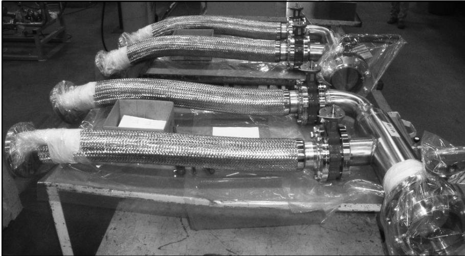
**Figure 3.6. Supply Header with Hoses for Endport Furnace**
