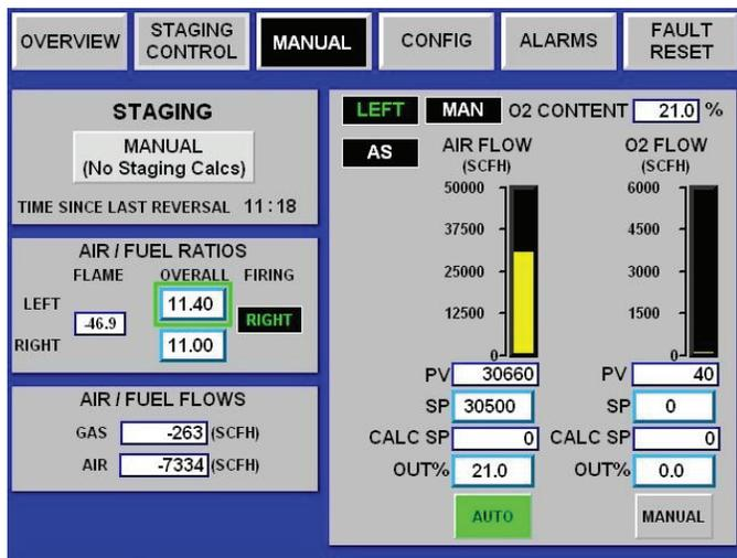
Figure 4.6. Manual Staging Control Screen
