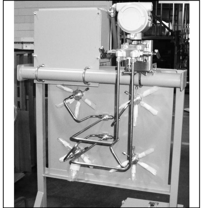
**Figure 3.5. Metering Panel Back**
