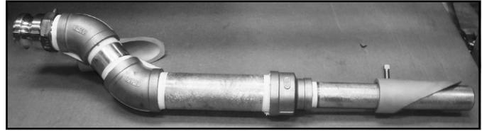
**Figure 3.2. Injector for Sideport Furnace**
