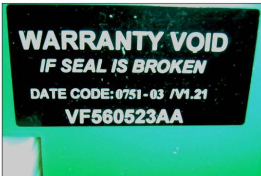
Some early units with the date code **0748-03 through 0801-03** may not be stamped on the front. If the label on the back of the unit shows -03 after the 4-digit date code, you can mark the 03 on the bottom front with a permanent marker to help with future identification.
