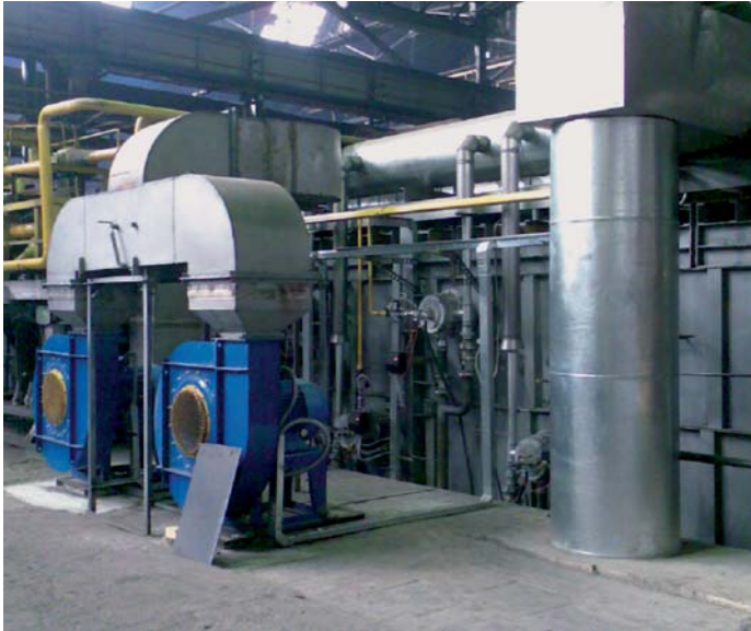
Fig. 4: View of the pusher-type furnace after revamping with ECO-MAX® self recuperative burner
