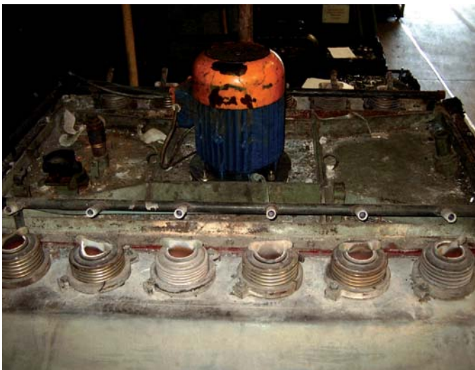
Fig. 5a/b: View of the roof of the hardening furnace before (left) and after (right) modernization with ECOMAX® self recuperative burners
