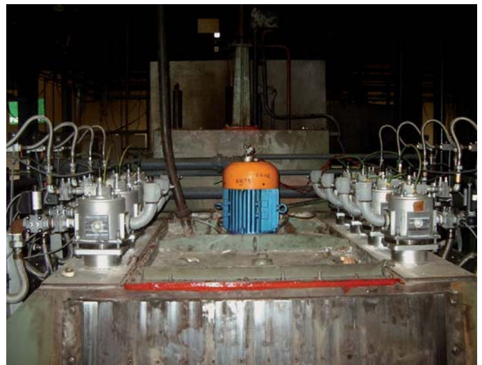
Fig. 5a/b: View of the roof of the hardening furnace before (left) and after (right) modernization with ECOMAX® self recuperative burners
