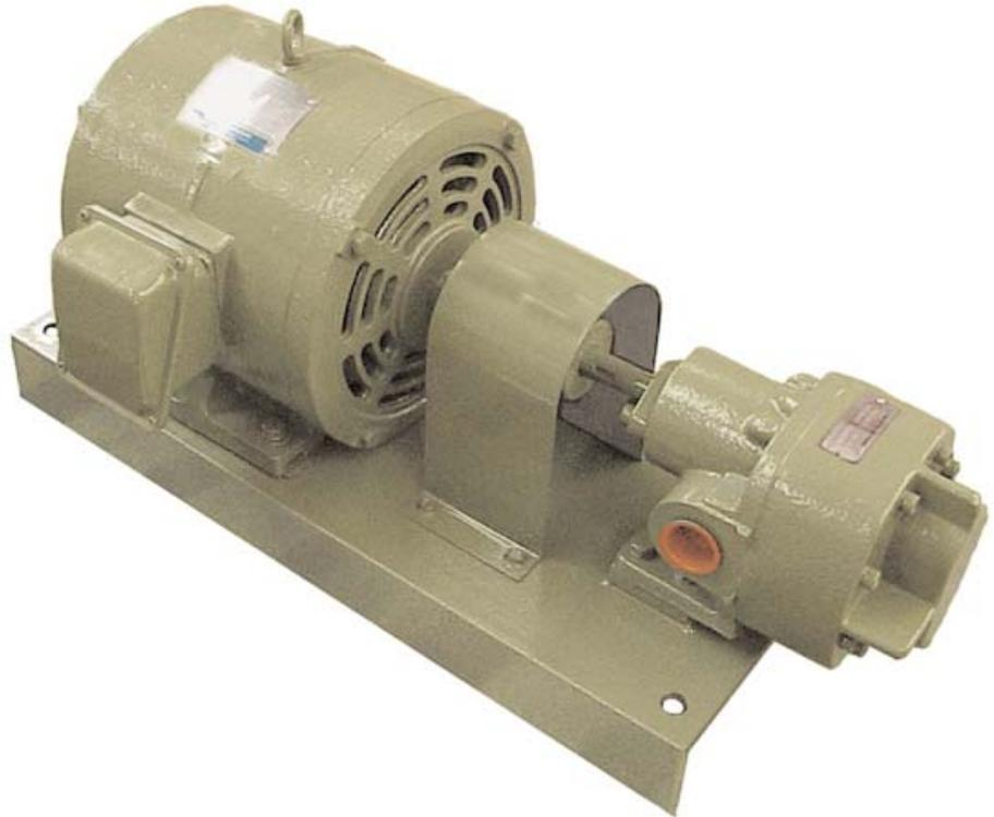
Hauck's RP series pump and motor sets are factory assembled units designed to meet your specific volume, viscosity, and discharge pressure requirements. Each set combines a positive displacement rotary gear pump with a suitable 'T' frame industrial electric motor mounted on a steel base. The motor and pump are matched to ensure that the requirements of the application are met with maximum efficiency.
