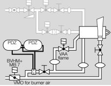
Control with butterfly valve and primary air valve (jump in capacity)
