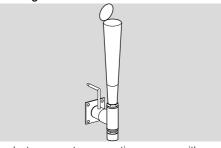
The eductor generates a negative pressure with a centrally positioned nozzle and thus draws the flue gases through the burner's heat exchanger. The EJEK is not supplied with the burner and must be ordered separately.
