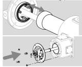
e Press the gas insert into position, secure the nuts by hand and then tighten them in a crosswise fashion using a torque of 20 Nm.
