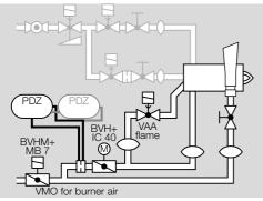
Control with two butterfly valves and a primary air valve (constant or variable capacity)
