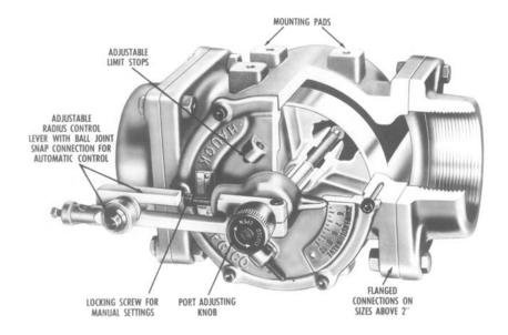
Figure 2. Adjustable Port Valve Cutaway Diagram
