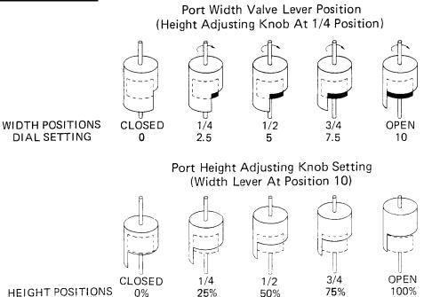
Figure 3. Illustration of Valve Height and Width Adjustments
