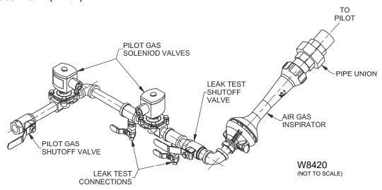
Figure 11. Gas Pilot Manifold
