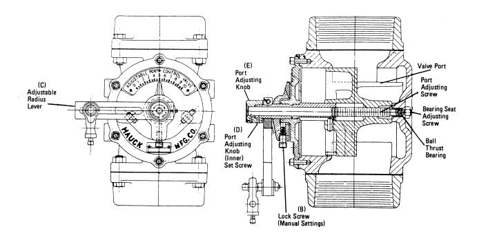
Figure 4. Adjustable Port Valve Diagram
