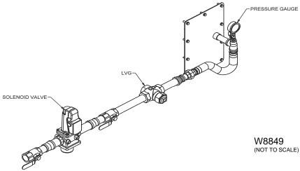
Figure 13. Center Gas Manifold
