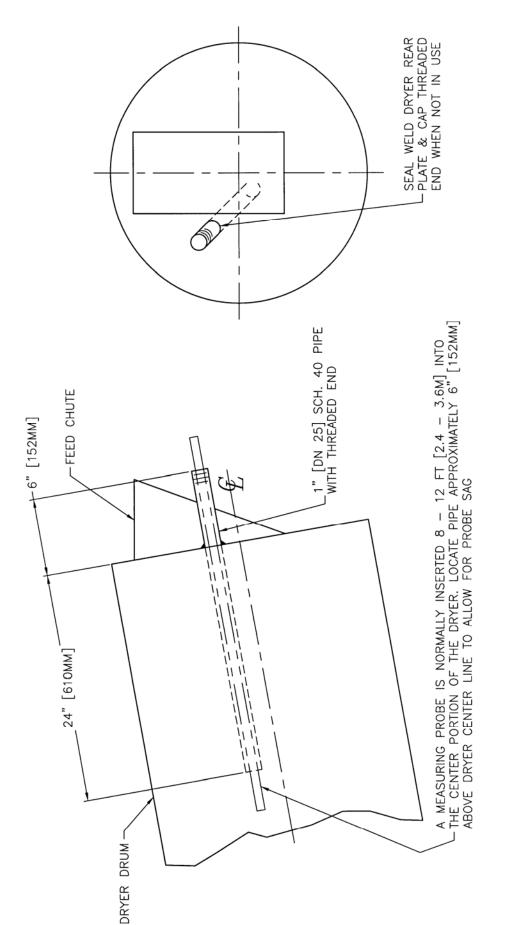
NOTE: 1. IF RECYCLE IN BEING USED, THE SAMPLE PIPE SHOULD BE AHEAD OF THE ENTRY 18 — 24" [460 — 610MM]
