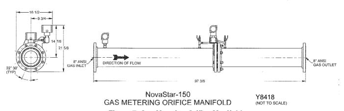
Figure 7. Gas Metering Orifice Manifold
