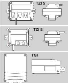
→ Position the ignition transformer right next to the burner (recommended ignition cable length: max. 5 m, recommended < 1 m).</p>
