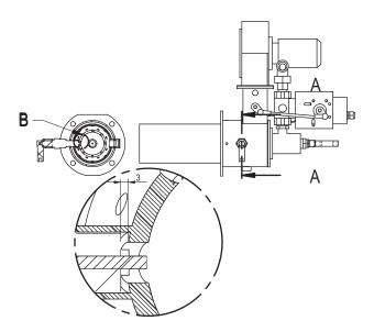
The spark ignitor can be mounted in 3 different positions on the burner housing: left, right and bottom (if the air inlet is on top). Spark ignitor replacement: insert the spark ignitor through the collar into the burner. Insert the spark ignitor in the cone bushing until its ceramic touches the cone - then retract the spark ignitor 0.12 inch to establish proper gap.
