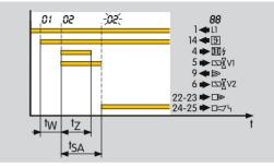
If, after a successful burner start, the automatic burner control unit does not detect a flame signal during the safety period on startup  $t_{SA'}$ , a fault lock-out will occur (fault signalling contact between terminals 24 and 25 closes). During the entire safety time on start-up  $t_{SA'}$ , the pilot gas valve V1 is open. The display blinks and indicates  $\square 2$ , see page 20 (Program status and fault messages).
