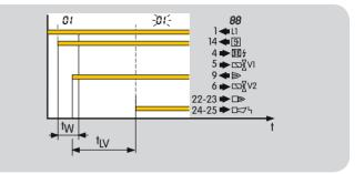
Flame simulation is an incorrect flame signal. If flame simulation is detected during start-up, the flame simulation delay time  $t_{LV}$  (max. 15 s) starts to elapse. If the flame simulation is discontinued during the flame simulation delay time  $t_{LV}$ , start-up can be initiated or operation continued. Otherwise, a fault lock-out occurs.
