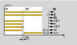
After a flame failure during operation, the IFD 450 will perform a fault lock-out within the safety time during operation  $t_{SB}$  (the safety time during operation  $t_{SB}$  is 1 second. The IFD 450 is available with a safety time of 2 seconds upon request). This involves closing the gas valves and disconnecting the power from the ignition transformer. The fault signalling contact closes and the display blinks and indicates  $\Box \Psi$  – see table "Program status and fault messages".
