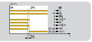
If the flame fails during operation, the valves are closed within the safety time  $t_{\text{SB}}. \label{eq:sb}$
