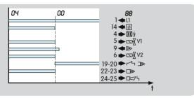
After switching off the start-up signal  $(\vartheta)$ , the valves close and the operation signalling contact (connection between terminals 22 and 23) opens. The burner switches off. The automatic burner control unit IFD checks in start-up position/ standby, whether an extraneous signal (flame simulation) is present. The display indicates the current program status  $\Box \Box$ .
