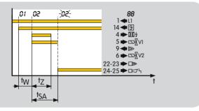
Once the start-up signal  $\vartheta$  has been applied, the waiting time  $t_W$  starts to elapse. During this time, a self-test is conducted to detect errors in internal and external circuit components. If no malfunction is detected, the burner will start up.
