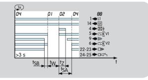
If the IFD 454 detects a flame failure after a minimum operating time of 3 seconds, the valves are closed and the operation signalling contact opened (terminals 22 to 23) within the safety time during operation  $t_{SB}$ .
