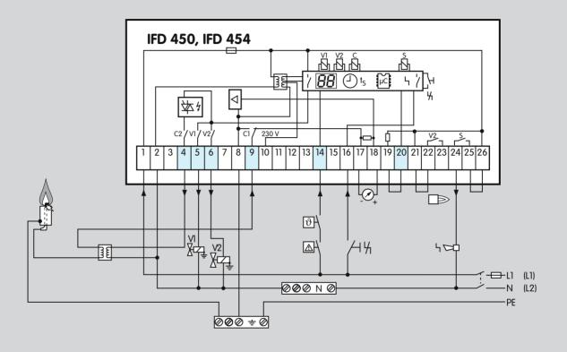
3.1.2 IFD 450, 454 with ionisation control in single-electrode
