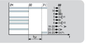
Flame simulation is signalled by at least one flame detector. The flame simulation delay time  $t_{LV}$  then starts to elapse. If the flame simulation is continued during the flame simulation delay time  $t_{LV}$  (max. 15 s), a fault lock-out will occur. The display blinks and indicates  $\boxed{F_{L}}$ .
