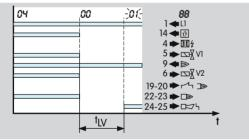
Once the burner has been shut down, flame simulation is signalled. The flame simulation delay time tLV then starts to elapse. If the flame simulation is continued during the flame simulation delay time  $t_{LV}$  (max. 15 s), a fault lock-out will occur. The display blinks and indicates  $\Box I$ .
