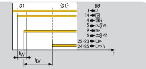
If flame simulation is signalled during start-up, the flame simulation delay time  $t_{LV}$  starts to elapse. If the flame simulation is discontinued during the flame simulation delay time  $t_{LV}$  (max. 15 s), the burner will start up. Otherwise, a fault lock-out occurs. The display blinks and indicates  $\square 2$ , see page 20 (Program status and fault messages).
