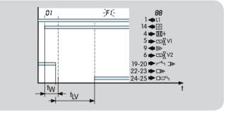
Flame simulation detected by at least one flame detector is signalled during start-up (no connection between terminals 19 and 20). The flame simulation delay time  $t_{LV}$  then starts to elapse. If the flame simulation is continued during the flame simulation delay time  $t_{LV}$  (max. 15 s), a fault lock-out will occur. The display blinks and indicates  $\overline{[F1]}$ , see page 20 (Program status and fault messages).
