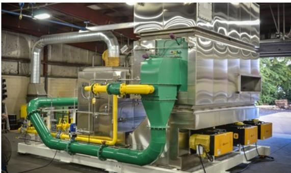
**Hauck NovaStar Ultra Low NO<sub>x</sub> Burner** for Asphalt & Aggregate Drying Application in the US. Commissioned in 2018.
