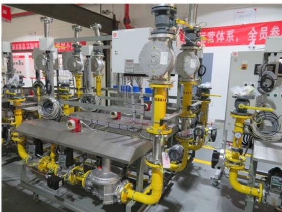
**Eclipse Packaged Burner System** for Heating Process Exhaust Application in China. Commissioned in 2017.
