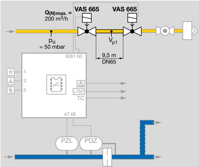
$$\text{Leckrate } Q_L = 200 \text{ m}^3/\text{h} \times 0,1 \% = 200 \text{ l/h}$$
