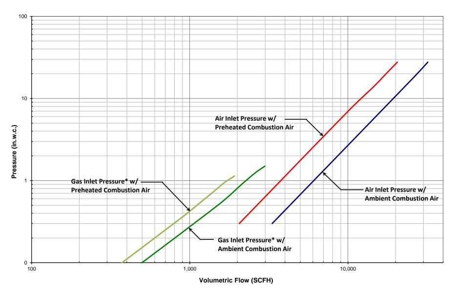
\*Note: Gas Inlet Pressure for BBG burner is not suitable for fuel flow measurement and is given for component sizing and reference only
