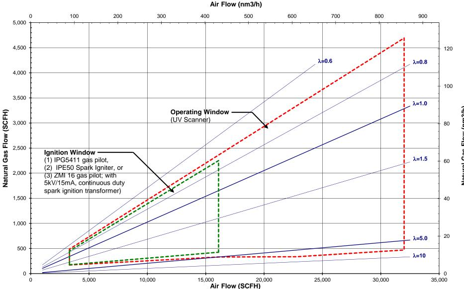
BBG 2004/3004 Operating and Ignition Window Natural Gas 1034 BTU/ft<sup>3</sup> (HHV Standard) / 10.21 kWh/nm<sup>3</sup> (LHV Metric), 0.59 S.G. and Ambient Combustion Air
