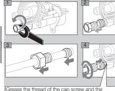
Grease the thread of the cap screw and the double-cone olive.
