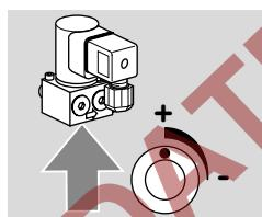
The flow rate can be set by turning the flow rate restrictor (4 mm/0.16" Allen screw)  $\frac{1}{4}$  of a turn. Flow rate: 10 to 100%.
