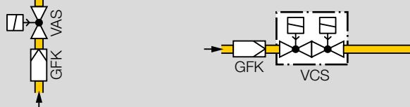
Installation position: black solenoid actuator in the vertical upright position or tilted up to the horizontal, not upside down.
