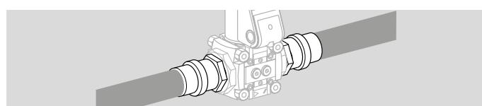
The seals in some gas compression fittings are approved for temperatures of up to 70°C (158°F). This temperature limit will not be exceeded if the flow through the pipe is at least 1 m³/h (35.31 SCFH) of gas and the maximum ambient temperature is 50°C (122°F).
