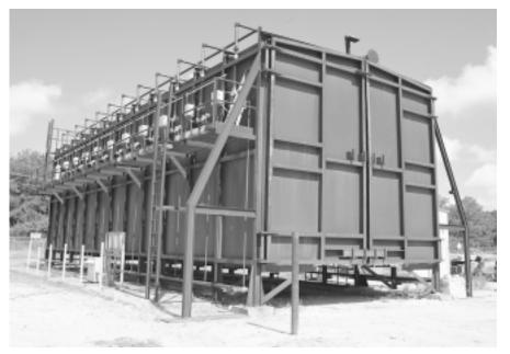
Designed for post-weld heat treating of large and heavy parts, SRS Wintergreen's new furnace incorporates 24 Eclipse ThermJet highvelocity, low NOx burners and Veriflame programmable burner monitoring system.
