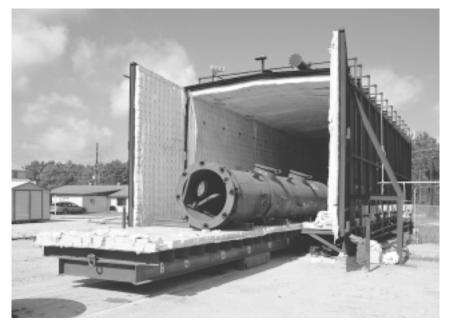
For heavy, bulky parts, this "inand-out," car-bottom design is a practical solution. Parts are loaded on a track-mounted car which is rolled into the furnace to form the bottom of the heating chamber. The furnace is 22 feet high by 25 feet wide by 60 feet long. Stress relieving is typically done at temperatures that range from 1050 to 2000 degrees F (566 to 659 degrees C), depending on the material and its chemistry.
