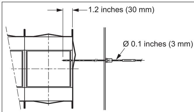
**Figure 5.2. Thermoelement Detail
