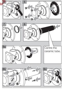
▶ Mounting flange and furnace flange must be flush.
