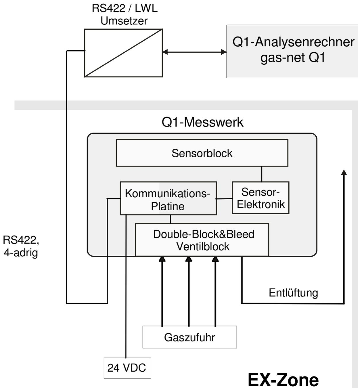
Figure 3: Schematic diagram of Q1 measuring unit and Q1 evaluation computer (gas-net Q1)
