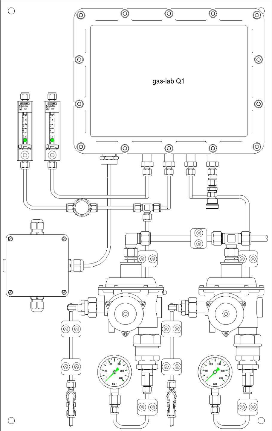
Figure 6: Mounting plate (example) with Q1 measuring unit, pressure controllers and connections
