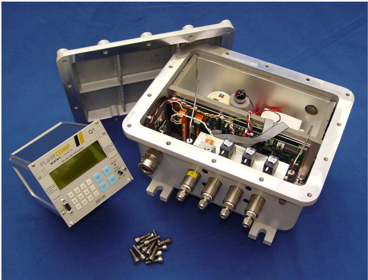
Figure 1: Q1 measuring unit (on the right) and Q1 evaluation computer (on the left)
