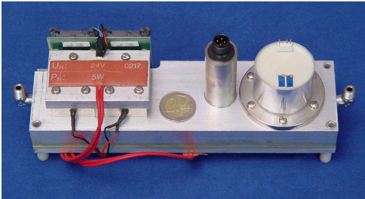
**Figure 2: Sensor system with two IR filter photometers, pressure transducer and thermal conductivity sensor**
