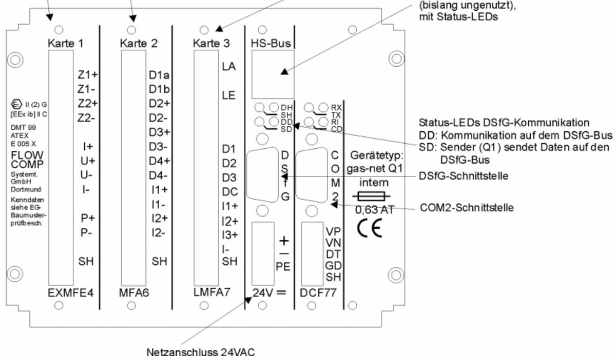
Figure 5: Rear view of the Q1 gas-net evaluation computer
