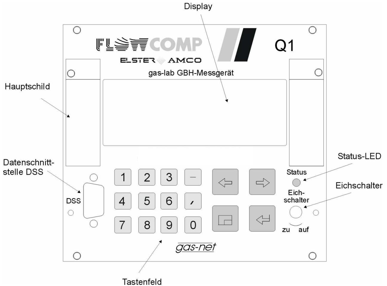
Figure 4: Front view of the Q1 gas-net evaluation computer
