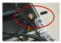
Screw the dummy plug into the former position of the antenna on the bottom side of the housing.
