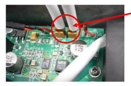
Fig. 6: Disconnect the modem backup batteries from the power supply.
