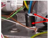
Secure the ferrite sleeve with cable ties.
