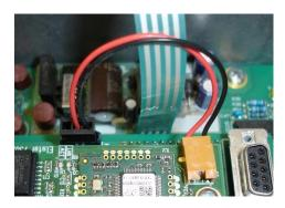
Fig. 19: Power supply to the Ethernet interface
