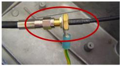
Pull the external antenna cable back outwards as far as possible, until the antenna adapter cable is lying against the inside of the cable gland.
