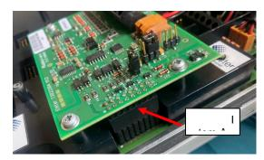
Secure the interface module to the black board cover using three plastic self-tapping screws (important: only one is supplied in the DL230 retrofit kit; two more must be ordered separately).
