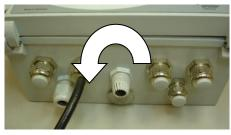
Screw in the cable gland on the lower right side of the housing.
