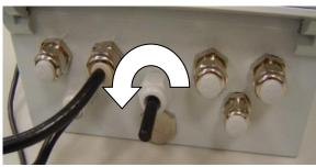
Remove the short antenna from the housing. Be careful not to stretch the antenna adapter cable when opening the housing cover.
