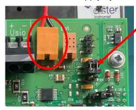
Both plug-in jumpers at the **top** or bottom position (the position is insignificant as the isolation is eliminated by the internal power supply unit)
