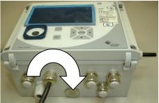
Reconnect the modem battery or the connection of the modem supply of the internal power supply on X3, "Battery", of the modem board.
