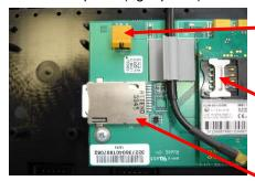
Connector for modem battery <u>or</u> internal power supply.
