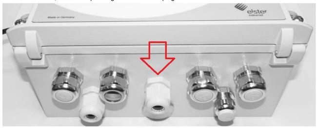
An A/F 20 wrench is required for the cable gland.
