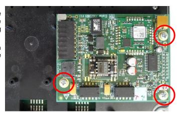
Once you have installed the Ethernet module in the EK280 ...
