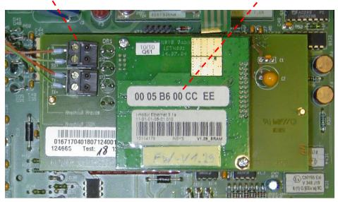
Fig. 13: INSYS Ethernet adapter in the FE260
