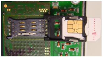
Fig. 8: open SIM card slot
