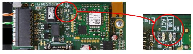
Fig. 21: "ACT" and "LILNK" LEDs on the iCE260 Ethernet interface
