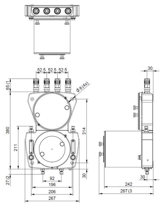
Fig. 5-1: Dimension drawing (with optional sand guard)
