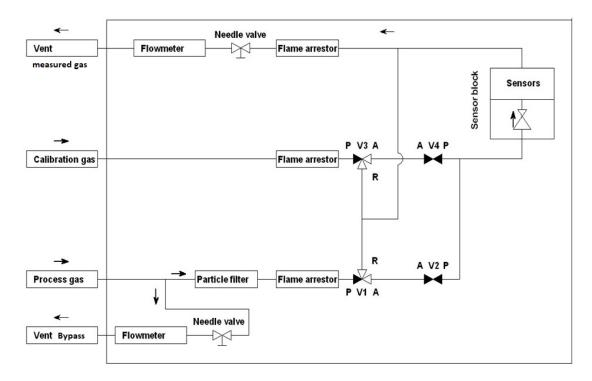
Fig. 4-2: Gas routes in the device
