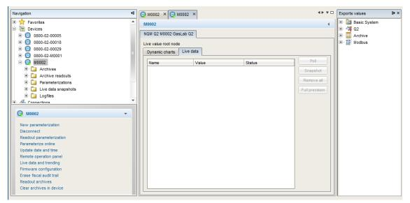
Fig. 8-33: Windows and tabs for "Live data and trending" function
