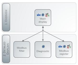
Fig. 7-47: Display – hierarchical structure
