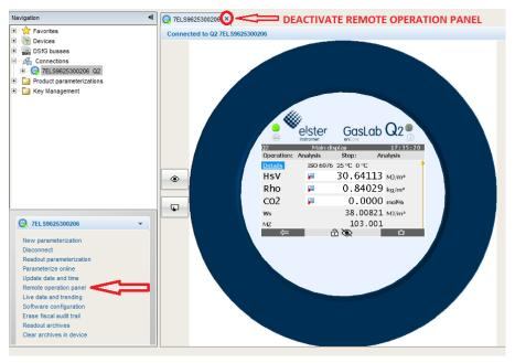
Fig. 8-52: View of the remote operation panel via enSuite
