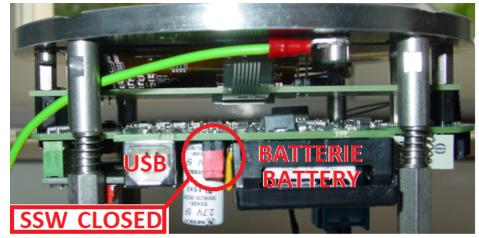
Fig. 6-2: SSW closed (jumper connected)
