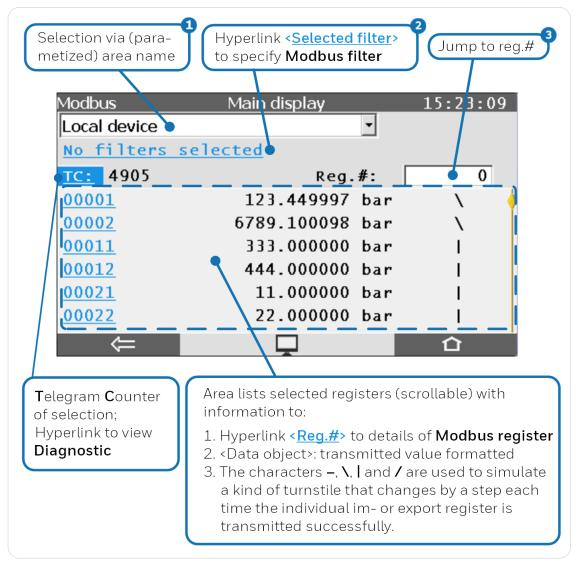
Fig. 7-48: Modbus Main display – example
