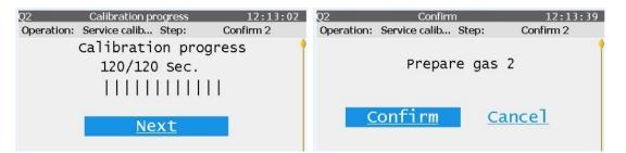
04 The procedure is repeated in the same way as for gas 1. After measuring the 2nd gas, **"Next"** appears again in the lower part of the display for switching to analysis mode. Select**"Next"**and restore the connections as they were before the service calibration! Conduct a tightness test.
