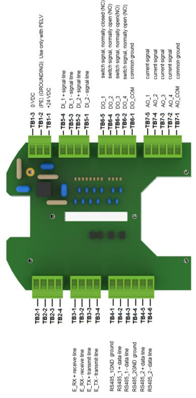
Fig. 5-6: Electrical connection assignment (circuit board)
