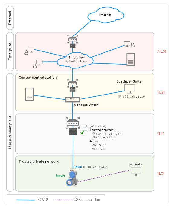
Fig. 2-3: Preventing unauthorized external access to enCore device – example with indication of security zones L0..L3 and higher according to IEC 62443
