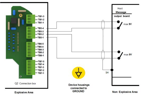
Fig. 5-9: Example connection of digital inputs
