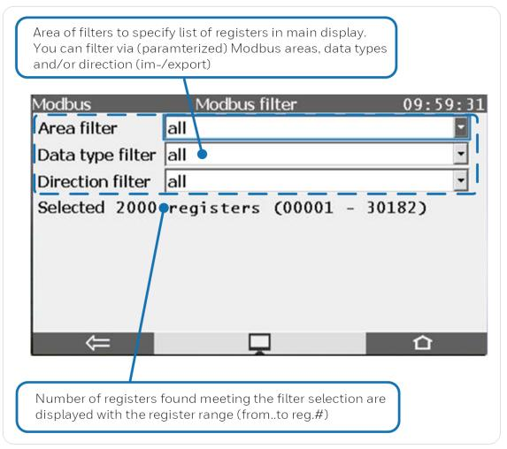
Fig. 7-49: Display **Modbus filter** – example
