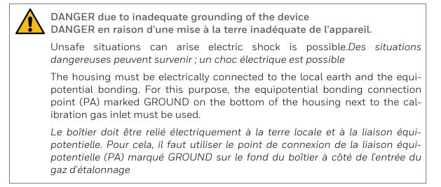
The conductor cross-section for grounding is least 6 mm<sup>2</sup>  $\triangleq$ 10 AWG (maximum 10 mm<sup>2</sup>  $\triangleq$ 8 AWG) copper conductor. The specified ground connection must be used with no modifications. The torque for the connection must not exceed 3.5Nm  $\triangleq$ 2.582 ftlb. If GasLab Q2 is mounted on a metal plate, the plate must be properly included in the grounding and the equipotential bonding system.
