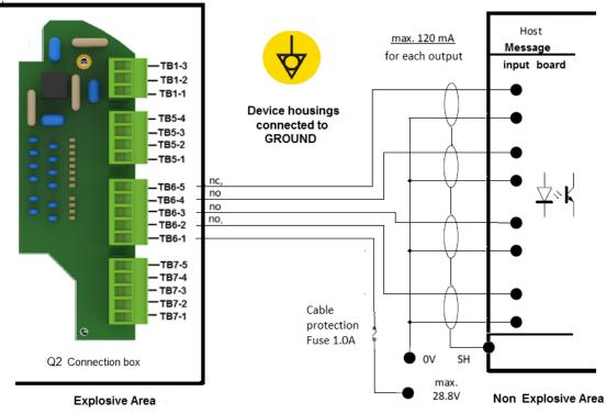
Fig. 5-10: Example connection of digital outputs
