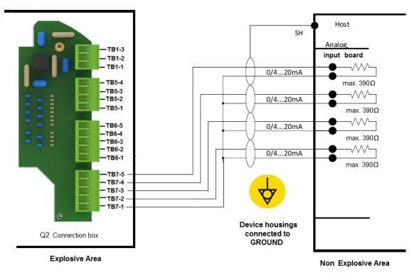
Fig. 5-11: Sample connection of digital outputs
