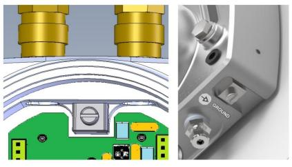
Fig. 5-4: Grounding inside connection box (FE) and outside of the device (PA)
