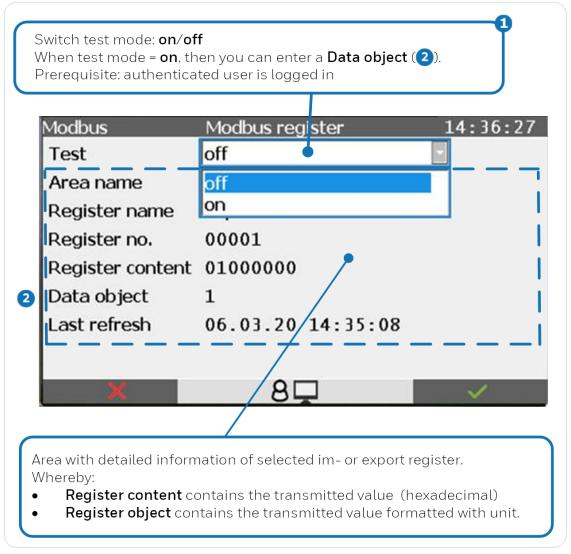
Fig. 7-51: Display **Modbus register** – example
