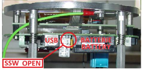
Fig. 6-3: SSW open (no jumper)
