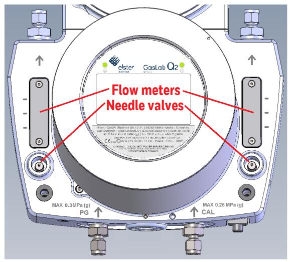
Fig. 3-3: Accessible elements of the instrumentation section
