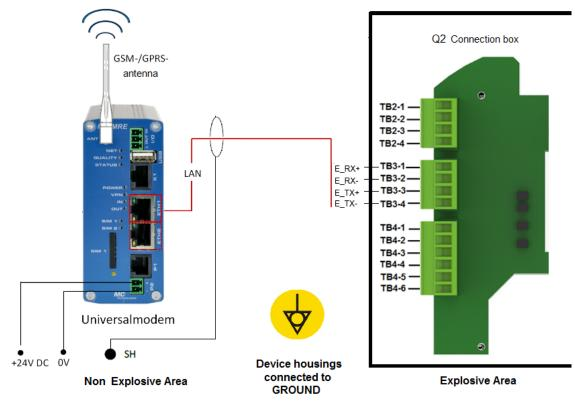
Fig. 5-7: Sample LAN/Ethernet connection (diagram)
