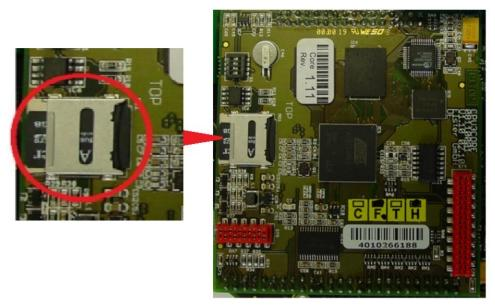
Fig. 10-3: CPU board with memory card
