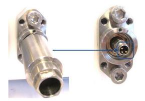
14. The valve at the bracket has to be mounted.
