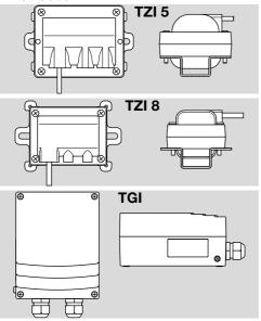
→ Position the ignition transformer right next to the burner (ignition cable length: max. 5 m, recommended < 1 m).
