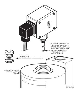
Fig. 1. Installing the 32004295-001 Closed Position Indicator Switch on the V4295A/ V4297A Valve.
