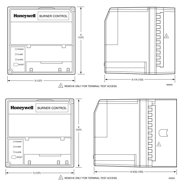
Fig. 1. Mounting dimensions of EC7823/RM7823 Relay Module and Q7800A,B Subbase in in. (mm).
