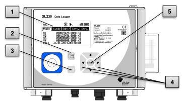
Fig. 17: Front panel of the DL230
