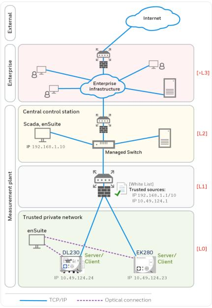
Figure 1: Router and firewall between the metering systems and control centre – example with indication of security levels L0..L3 and higher according to IEC 62443
