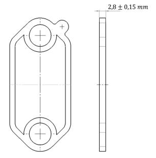
Figure 3 Moisture Protection Gasket drawing in doc. 73025161
