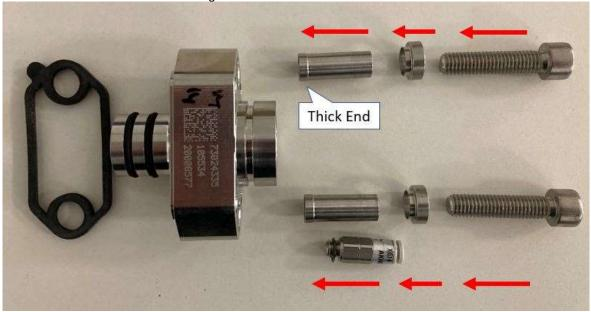
Figure 17: correct assembly of mounting bolts and rivets
