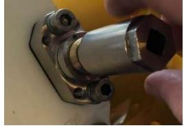
Figure 23: reinserting the brass lock inner nut
