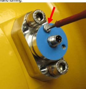
Figure 6: unscrew the alignment disc bolt
