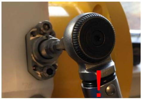
Figure 25: reinstall the brass lock inner nut and apply 12 Nm torque
