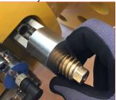
5. Attach nut to the spindle
