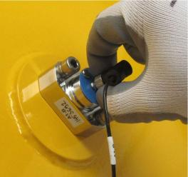
Figure 4: Disconnecting transducers
