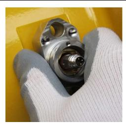
Figure 12: removing the transducer mounting set from the meter body
