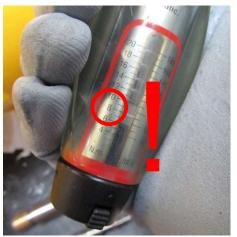
Figure 21: tightening the transducer mounting bolts to 8 Nm
