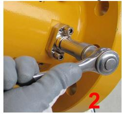
Figure 8: Loosening the brass lock inner nut
