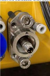
Figure 22: reinserting the transducer shaft
