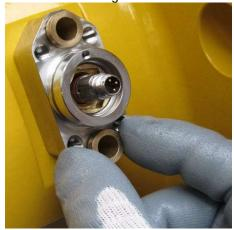
Figure 10: Removing the rivets
