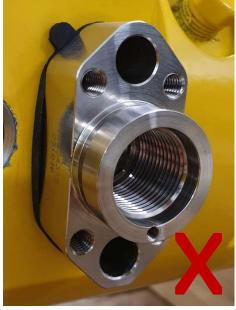
Figure 20: Correct placement of the Moisture Protection Gasket: good (left) vs. bad (right)
