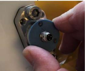
Figure 24: aligning the transducer
