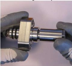
Figure 13: removing the brass lock inner nut
