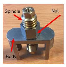
Figure 15 Retraction Tool USM Bracket Serie 6
