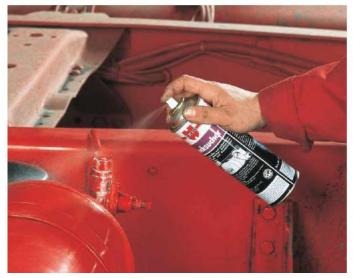
Figure 38. Gas leak detection agent
