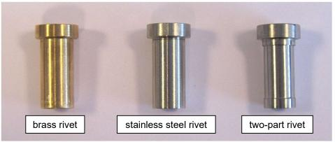
Figure 11: Types of rivets used in the mounting bracket
