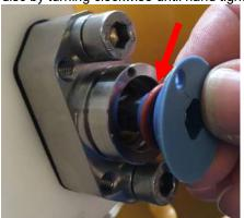
Figure 27: reinstalling the alignment disc and bolt
