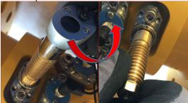
2. Attach other side of the spindle to the transducer and retract transducer out of the bracket
