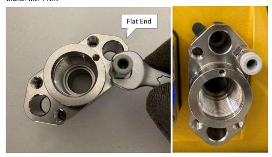
Figure 19: correct positioning of the Check Valve on the transducer bracket
