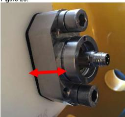
Figure 26: pull and push the mounting bracket to ensure it's free to move a bit
