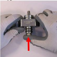
Figure 14: pushing the transducer out of the mounting bracket
