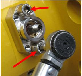
Figure 9: Unscrewing the transducer mounting bolts
