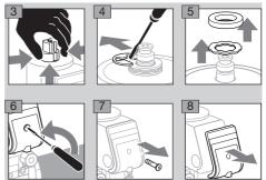
Remove the M20 cable gland or other type of connection.
