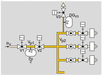
The valves and the pipework between the valves are tested.
