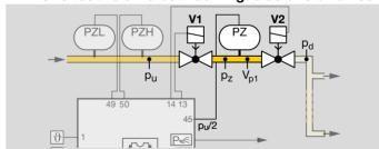
The tightness control checks the tightness of the test volume  $V_{\text{D1}}$  between gas solenoid valves V1 and V2.
