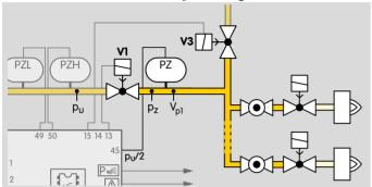
The tightness control checks the system tightness of the test volume  $V_{p1}$  between the central shut-off valve V1, relief valve V3 and the burner valves. The opening times of the relief valve V3 and the shut-off valve V1 are identical.
