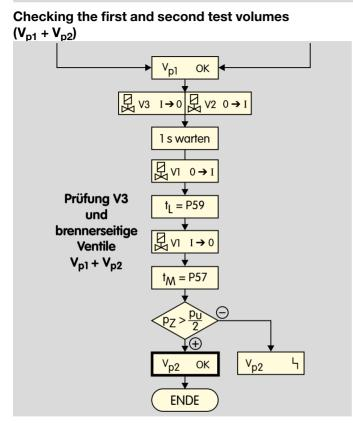
To check the test volume  $V_{p2}$ , relief valve V3 is closed and valve V2 is opened. The two test volumes  $V_{p1}$  and  $V_{p2}$  are connected to each other. After a waiting time of 1 s, valve V1 opens for the opening time  $t_L$  set in parameter 59. Valve V1 then closes and the measurement time set in parameter 57 starts to elapse, see page 107 (12.5.7 Measurement time Vp1 and Vp2). After the measurement time has elapsed, the tightness control checks pressure  $p_7$ . If
