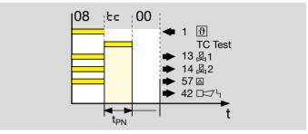
After the furnace has been shut down, the FCU starts testing the tightness of the gas solenoid valves and pipework between the valves. After the tightness has been checked successfully, the next furnace start is enabled as regards the tightness criteria.
