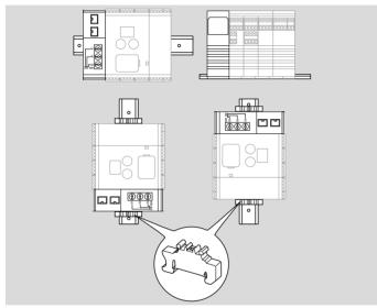
If the DIN rail is aligned vertically, end clamps are required (e.g. Clipfix 35 by Phoenix Contact) to prevent the control unit from slipping.
