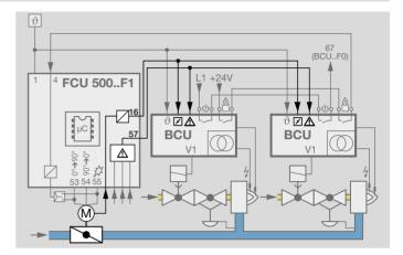
A corresponding circuit design between the FCU and the BCUs ensures that the burners can only start if the safety interlocks and the LDS output are active.
