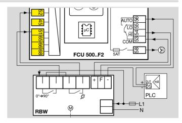
The RBW actuator reports that it has reached the position for maximum capacity via a signal to terminal 51. The actuator reports that it has reached the position for minimum capacity via a signal to terminal 52. The simultaneous activation of terminals 51 and 52 results in a fault lock-out of the FCU.
