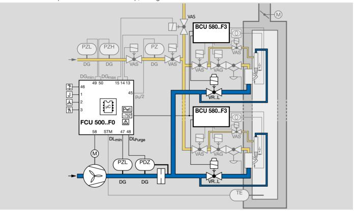
The capacity control function provided by the FCU 500..F1/F2 and FCU 505..F1/F2 allows an additional central actuator or a frequency-controlled fan to be controlled and moni-
