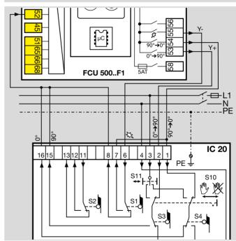
Parameter 75 = 2: MIN. to MAX. capacity; standby in CLOSED position. The control range while the burner is operating is between the positions for minimum capacity (S2) and maximum capacity (S3). The burner is ignited in the position for ignition capacity (S1). When the burner is switched off, the actuator is moved to the closed position (S4).
