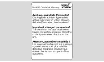
Affix on the connection diagram of the FCU 500, FCU 505 following changes to device parameters set at the factory.
