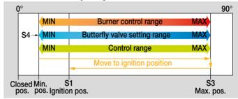
The control system is enabled during operation via the controller enable output (terminal 56). During the controller enable procedure, the actuator can be adjusted infinitely between the positions for maximum and minimum capacity using its analogue input (terminals 17 and 18). There is no timeout active in this case.
