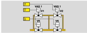
2. System leak tightness check with one test volume and pressure reduction using relief valve (parameter 53 = 2):
