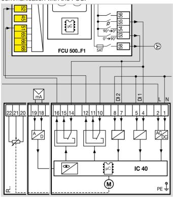
The positions for maximum capacity and ignition capacity can be set using the actuator. Terminal 51 checks whether the position for maximum capacity has been reached.
