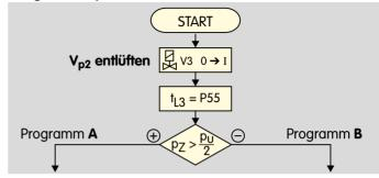
At the start of the tightness test, the relief valve V3 is opened to reduce the pressure of the test volume  $V_{p2}$  to around atmospheric pressure. The opening time for V3 can be defined using parameter 55, see page 107 (12.5.5 Opening time relief valve V3). The tightness control queries the pressure  $p_Z$  using the external pressure switch to check the first test volume. If pressure  $p_Z > p_U/2$ , program A starts. If pressure  $p_Z < p_U/2$ , program B starts.
