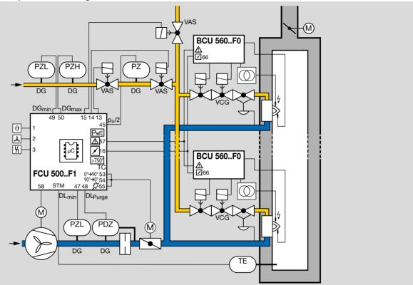
The centrally checked safety functions such as pre-purge, setting the valve to ignition position via a butterfly valve control system, tightness test, flow detector and pressure switch check ( $gas_{min.}$ ,  $gas_{max.}$ ,  $air_{min.}$ ) are provided by the FCU 500. The capacity can be adjusted continuously by activating the control element (analogue or 3-point step signal).
