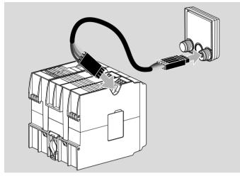
Cables for signalling and telecommunications systems are recommended for wiring the supplied plug connectors: cable length: max. 10 m, 4-pin, min. 0.25 mm² (AWG 24), max. 0.34 mm² (AWG 22).
