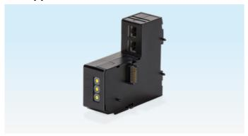
The bus module BCM 500 is used as a communication interface for devices of the BCU/FCU 500 product family for connection to a fieldbus communication system (Profinet or Modbus TCP). Networking via the fieldbus enables the FCU or BCU to be controlled and monitored by an automation system (e.g. PLC).
