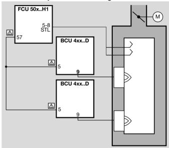
If the limit value of the safety temperature limiter is exceeded (excessive temperature in furnace), the FCU will perform a lock-out. The fault lock-out cannot be reset until the temperature falls below the STL limit value and the defined temperature hysteresis.
