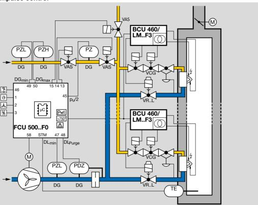
For processes which require a turndown of more than 10:1 and/or those which require heavy circulation of the furnace atmosphere to ensure a uniform temperature, e.g. heat treatment furnaces operating at low and medium temperatures in the metallurgical industry.
