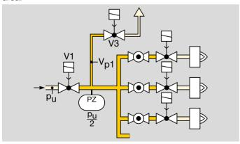
Parameter 53 = 3:  $V_{p1} + V_{p2}$ ; pressure reduction via V3.
