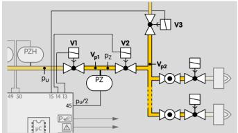
The test volumes  $V_{p1}$  and  $V_{p2}$  (gas solenoid valves V1 and V2, relief valve V3, the burner valves and the pipework) are checked to test the system tightness of the entire gas inlet section.
