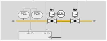
A signal is sent to the FCU via the POC switch on the gas solenoid valve on the inlet side before burner start-up stating that the valve is closed. After burner start-up, the signal must drop out to indicate to the FCU that the valve is open.
