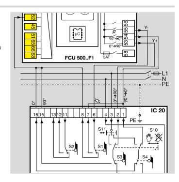
Parameter 75 = 4: MIN. to MAX. capacity; standby in position for MIN. capacity; burner quick start.
