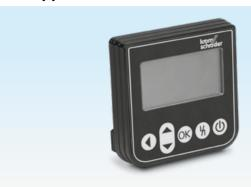
The OCU is an external operator-control unit which can be connected to a control unit of the FCU 500/BCU 500 series. The external operator-control unit OCU is installed in the door of a control cabinet. Thus, the control cabinet does not need to be opened to read out process values, statistics, flame signal intensities or parameter values, to change settings on the OCU or to control or adjust connected valves in Manual mode.
