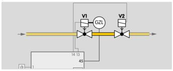
By checking the closed position using the proof of closure function, the FCU complies with the requirements of NF-PA 85 (Boiler and Combustion Systems Hazards Code) and NFPA 86 (Standard for Ovens and Furnaces).
