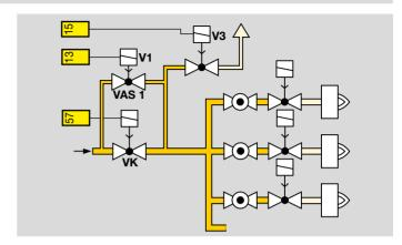
3. System leak tightness check with two test volumes and pressure reduction using relief valve (parameter 53 = 3):
