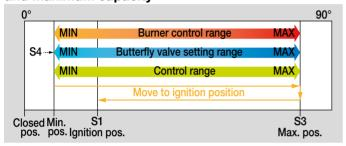
The control system is enabled for operation via the controller enable output (terminal 56). During the controller enable procedure, the actuator can be adjusted infinitely between the positions for maximum and minimum capacity by an external three-point step controller. There is no timeout active in this case.
