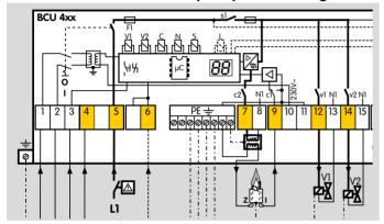
BCU 4xx without power management via phase (L1): in the event that a higher output current is required, the output current can be increased by means of a contact multiplier using 3 contactors.
