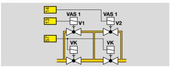
On condition that the gas volume which flows into the combustion chamber is no larger than 0.05% of the maximum flow rate, the bypass valves may be open for longer than the 3 s permitted by the standard (EN 1643:2000). The required volume limit can be achieved by fitting a restrictor or orifice, for example. The opening time to be set is then calculated on the basis of this restrictor or orifice.
