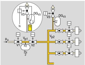
A pressure switch  $DG_{V3}$  can be connected between V3 and terminal 15 of the FCU for the controlled pressure reduction of the test volume  $V_{\rm p2}$  via a relief valve.
