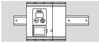
If the DIN rail is aligned vertically, end clamps are required (e.g. Clipfix 35 by Phoenix Contact) to prevent the FCU 500, FCU 505 from slipping.
