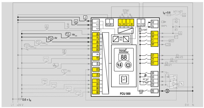
On FCU 500, actuation of the input at terminal 2 activates the controlled air flow function. The fan (terminal 58) is started in standby (with no start-up signal). Air is fed to the combustion chamber, e.g. for cooling.
