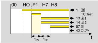
The FCU starts testing the tightness of the gas solenoid valves and pipework between the valves parallel to the pre-purge time. The gas line is always safeguarded by a gas solenoid valve during this check. When pre-purge is finished and the tightness has been checked successfully, the safety valves for operating the system are opened after the safety interlocks have been enabled.
