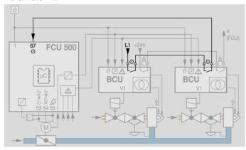
The terminal can be assigned the function "BCU ready". The FCU is informed via terminal 67 that there are sufficient burner control units for operation. If there is no "BCU ready" signal, the FCU will perform a safety shut-down or fault lock-out, depending on the function selected in parameter 72.
