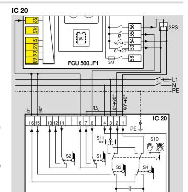
The positions for maximum capacity, ignition capacity and minimum capacity can be set using the actuator. It is checked whether the relevant position has been reached using terminal 52. If the position is not reached within the timeout time of 255 s, the FCU will display fault message Rc, Ro or Ri (minimum, maximum or ignition capacity not reached), see page 70 (11 Fault messages).
