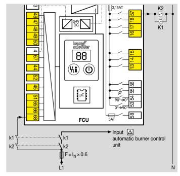
Use contactors with forced-guided contacts in this case. The two NC contacts in the contactors are connected in series to the safety interlock check signal input (terminal 68); the contacts must be protected with a factor  $\leq$  0.6 x I<sub>N</sub>, see page 117 (14.3.2 Safety current inputs).
