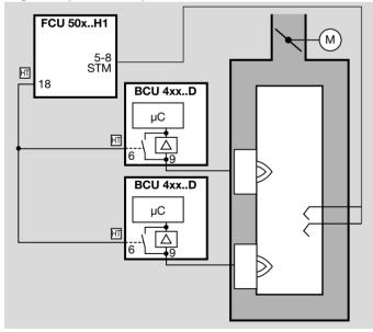
High temperature mode is reactivated as soon as the temperature exceeds the STM limit value and the defined temperature hysteresis.
