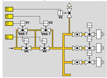
Current rating of safety interlock output (terminal 57): max. 0.5 A, see also page 122 (14.5.1 Safety interlock output in the case of higher power requirement).
