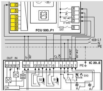
The positions for minimum capacity, maximum capacity and ignition capacity can be set using the actuator. When the appropriate position has been reached, this information is signalled back via terminal 52.
