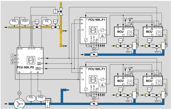
The FCU 500 (furnace FCU) performs central tasks such as checking the safety interlocks, fan control, system leak tightness check and pre-purge.
