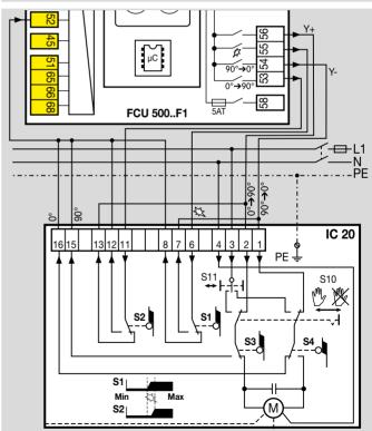
Parameter 75 = 5: IGNITION to MAX. capacity; standby in CLOSED position; burner quick start.
