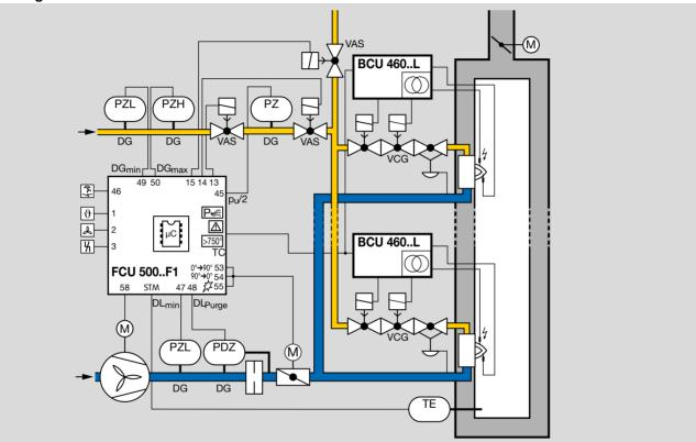
For processes that do not require heavy circulation in the furnace, e.g. aluminium smelting furnaces.
