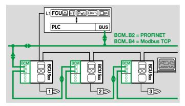
The basic function of Profinet and Modbus TCP is the exchange of process and required data between a controller (e.g. PLC) and several distributed devices (e.g. BCU/FCU/FDU).
