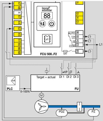
The FCU bridges the connections at terminals 53 and 54 (COM – HI bridge) for pre-purge. The frequency converter sets the fan to the speed for maximum capacity with a timeout of 255 s.
