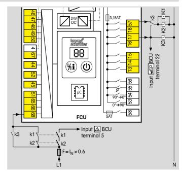
Use contactors with forced-guided contacts in this case. The two NC contacts of K1 and K2 in series and parallel to them the NO contact of K3 are connected to the safety interlock check signal input (terminal 68). The contacts must be protected with a factor of  $\leq 0.6 \times I_N$ , see page 117 (14.3.2 Safety current inputs).
