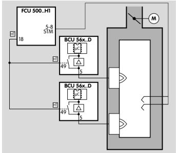
In high temperature systems (temperature > 750°C), the flame may be controlled indirectly via the temperature. As long as the temperature in the furnace chamber is below 750°C, the flame must be controlled by conventional methods.
