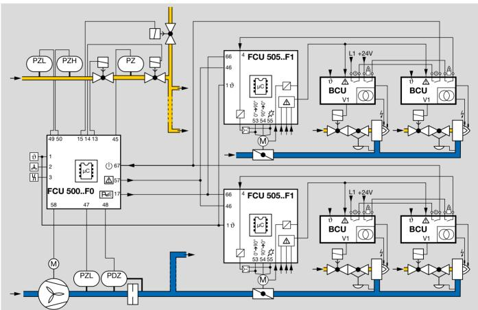
For furnace zone control, one FCU 500 is used to control the furnace and several FCU 505 are used to control the individual modulating zones (FCU 505..F1 or FCU 505..F2).
