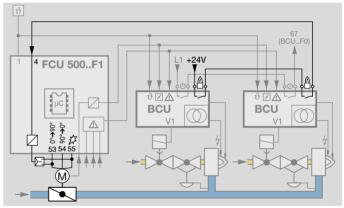
To ensure that the furnace control unit does not endlessly wait for the enable signal, a time (0 to 60 min.) can be defined using parameter 47 by which the burners must reach their operating position. If no feedback signal is received during this time, the FCU performs a fault lock-out. The time does not start until the minimum enable time has elapsed.
