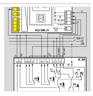
Parameter 75 = 3: IGNITION to MAX. capacity; standby in CLOSED position.
