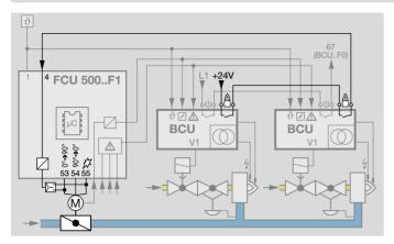
Depending on parameter 40, actuators IC 20 or IC 40, an actuator with an RBW interface or a fan controlled by a frequency converter can be actuated via the outputs for central capacity control, see page 89 (12.4.9 Capacity control).
