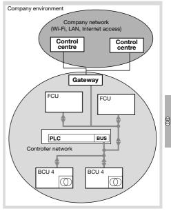
One possible example of a secure gateway would be a VPN set-up with defined authorized users. The following should be noted to ensure that a con-
