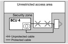
Protected and unprotected wiring
