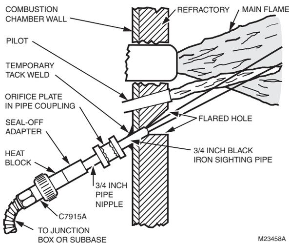
Fig. 9. Mounting C7915A Infrared Flame Detector (and accessories).
