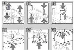
> The cylinder pin in the drive shaft must be locked in the coupling.
