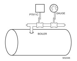
Fig. 3. Connecting P7911C PressureTrol® Controller to steam boiler.
