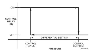
Fig. 6. P7911C on/off control function versus pressure.
