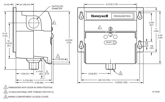
Fig. 1. Approximate dimensions of P7911C PressureTrol® Controller in in. (mm).
