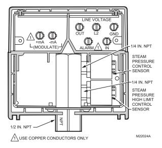
Fig. 4. P7911C PressureTrol® Controller.
