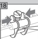
For longer burners, slide the other guide lugs against the retaining plate. Hand tighten the screw.
