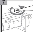
Loosen the screw of the retaining plate by turning it approx. 3 turns.
