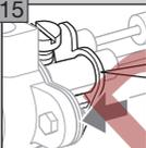
Slide the rear guide lug as far as it will go in the direction of the burner body. Hand tighten the screw.
