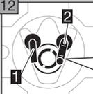
Align the spark electrode **1** and the flame rod **2**.
