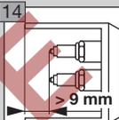
Slide the rear guide lug as far as it will go in the direction of the burner body. Hand tighten the screw. > 9 mm
