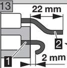
Adjust the spacing of the electrode tips. 22 mm, 2 mm.
