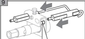
For correct positioning, slide in the electrodes until the projection of the retaining plate engages into the groove.
