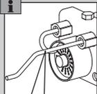
When sliding in the electrodes, ensure they are aligned.
