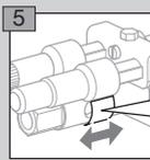
The air slide is open on delivery. Only close the air slide if the burner flame is not stable.
