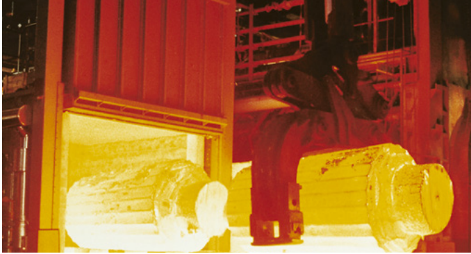
Bogie hearth forging furnace in the metallurgical industry
