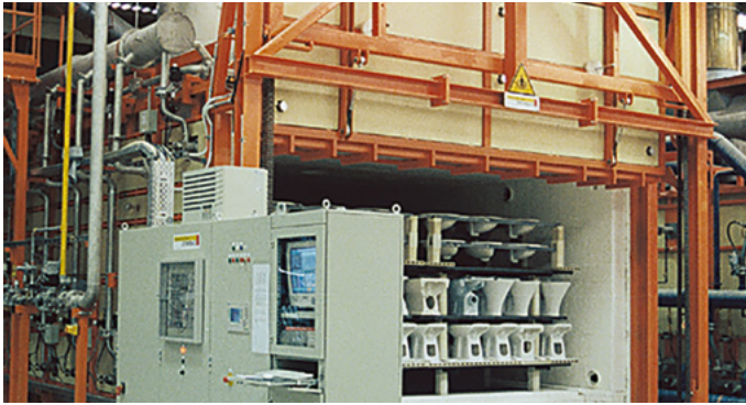
Intermittent shuttle kiln in the ceramics industry
