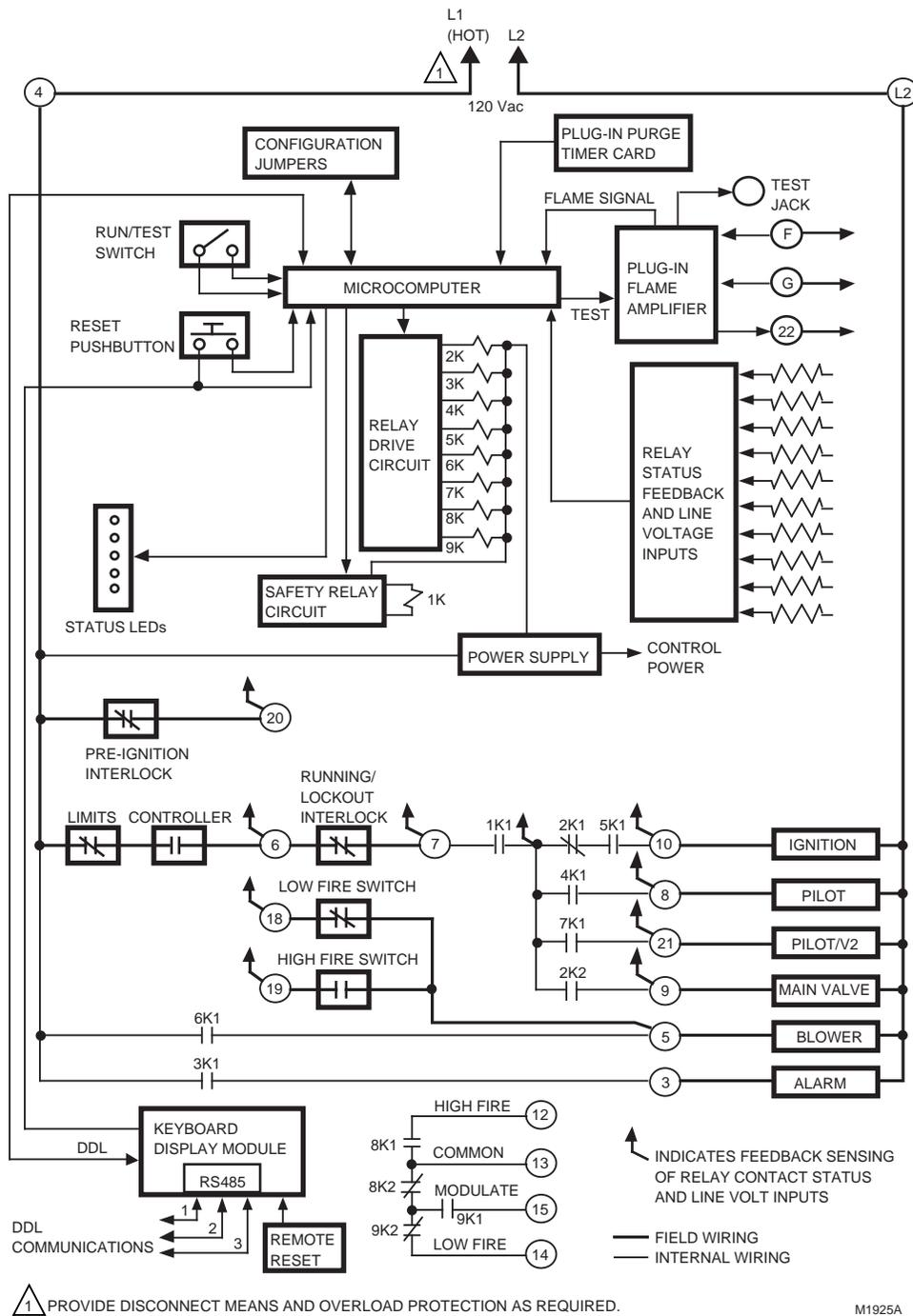
Fig. 5. Internal block diagram of the RM7800L (See Fig. 7, 8, 9, 10 or 11 for detailed wiring instructions).
