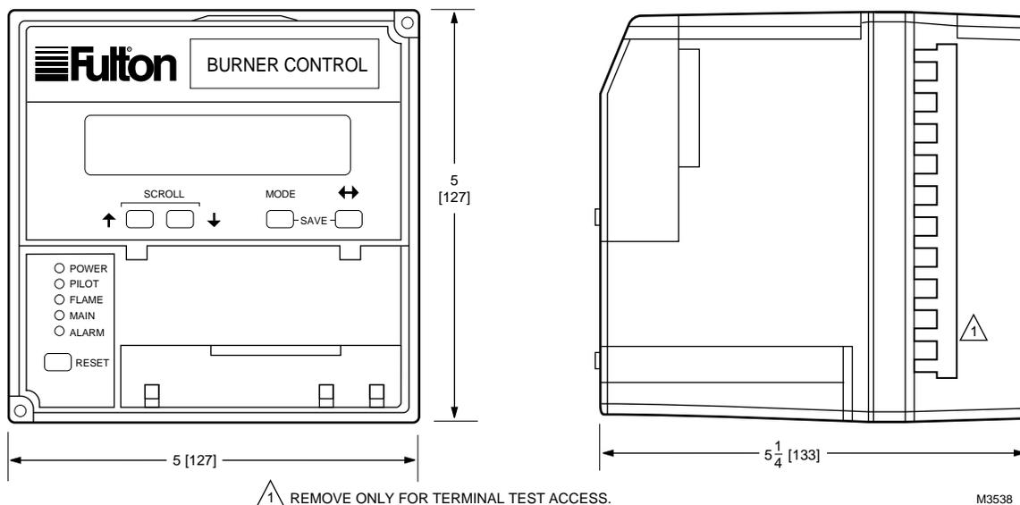
**Fig. 1. Mounting dimensions of RM7800 Relay Module and Q7800 Subbase in in. (mm).**
