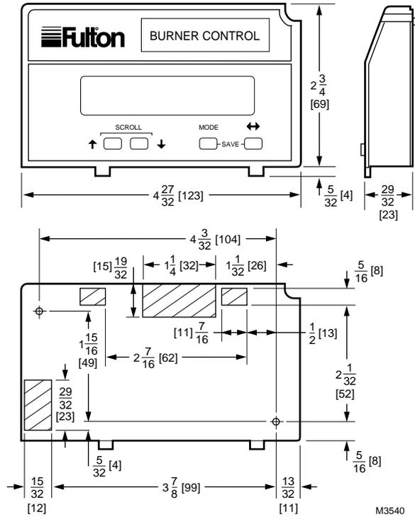
Fig. 2. Mounting dimensions of Keyboard Display Module in in. (mm).
