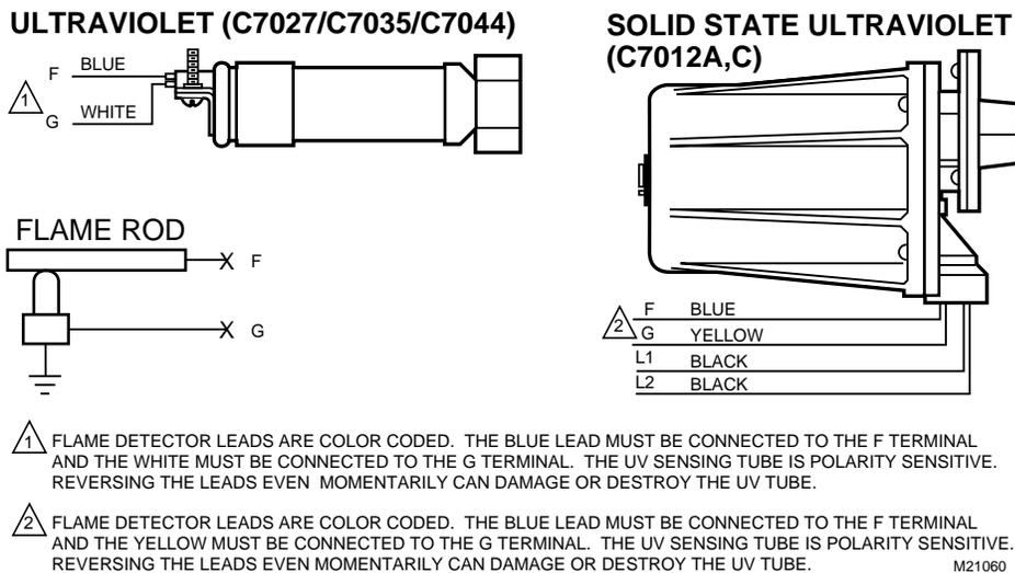
Fig. 19. Flame detector wiring.
