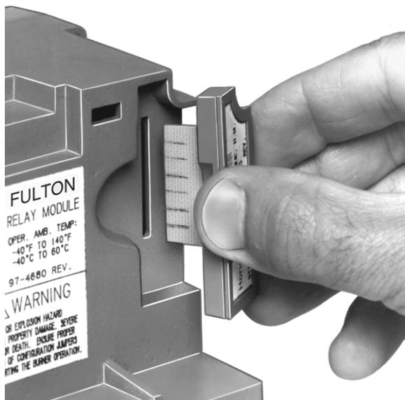
Fig. 12. ST7800 Purge Card installation.
