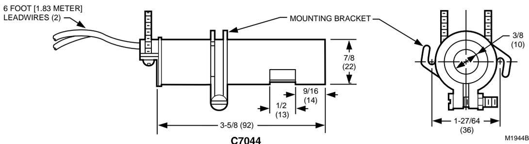
Fig. 4. Ultraviolet detectors.
