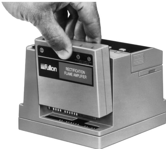
Fig. 18. Flame signal amplifier mounting.
