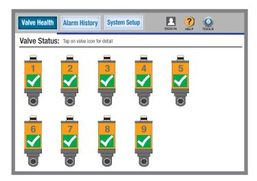
**Green** check mark indicates that the valve has PASSED and is operating properly; **Yellow** exclamation point indicates that the valve's performance is in ALERT mode and is degrading; and a **Red** "X" indicates the valve has FAILED the partial stroke test.
