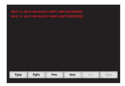
View alarm history (list of alarms). Captures all alarms, the dates of the alarms, and valve testing information when either a soft "alert" alarm or a hard "failure" alarm is triggered. The system will track all alarm instances over the life of the valve.
