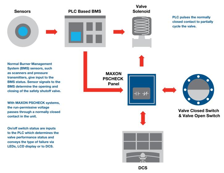
The MAXON PSCHECK technology is an IEC 61511 SIL2 certified diagnostic system that along with Maxon's Series 8000 valves helps meet SIL3 compliant Safety Instrumented System (SIS) performance requirements.
