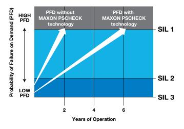
Increased length between valve maintenance while maintaining SIL 2.
