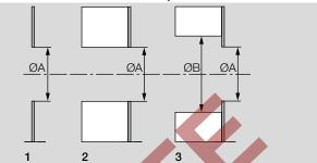
**Sketch 1 :** sheet metal combustion chamber/furnace without internal insulation. Flange/opening internal diameter shall be ØA
