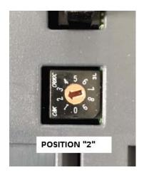
Amplifier Module Position Setting Switch
