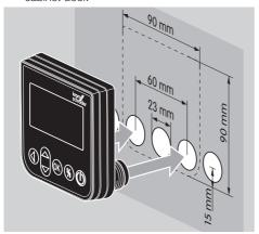
3 Screw the nuts on to the threaded adapters so that the OCU is firmly attached to the door.
