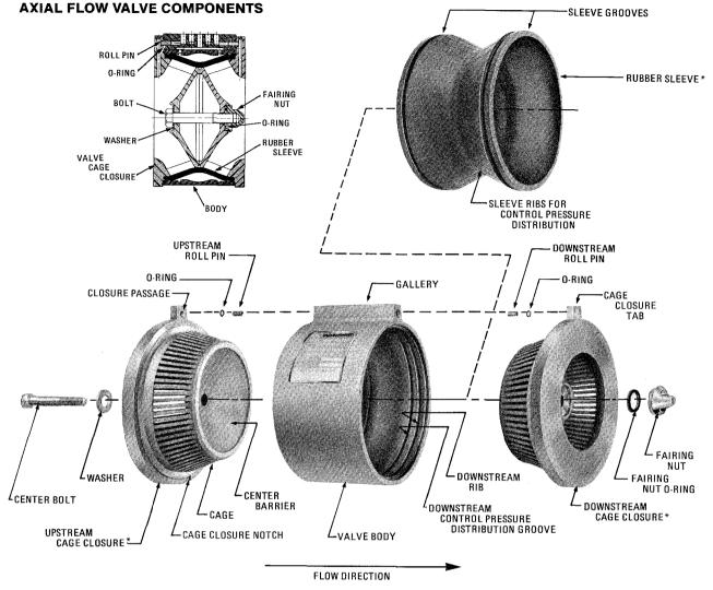
\*CAGE CLOSURES ARE INTERCHANGEABLE. RUBBER SLEEVE CAN BE INSTALLED IN EITHER DIRECTION. THE AXIAL FLOW VALVE IS CAPABLE OF BI-DIRECTIONAL FLOW CONTROL.
