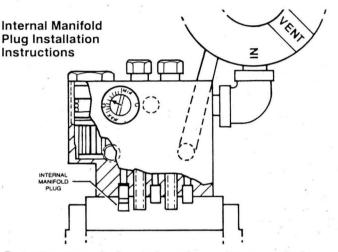
Downstream monitoring and passive upstream monitoring applications require the use of an internal inlet plug to block the pilot supply and to prevent pressure build-up in the intermediate piping between the two Axial Flow Valves. This plug is available as a retrofit kit; order Kit Number 74036K001
