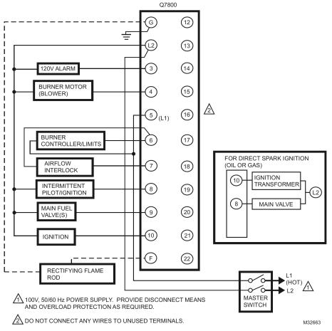
Fig. 7. Wiring the RM7895E, F Relay Module.
