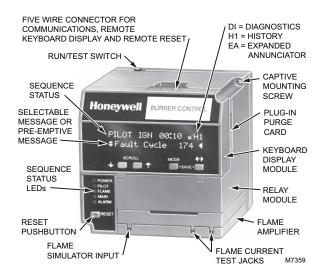
Fig. 11. Relay Module and associated system components.
