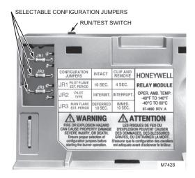
Fig. 12. Selectable site-configurable jumpers.
