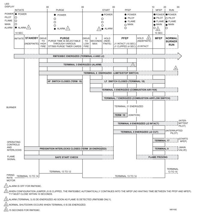
Fig. 8. RM7838B,C Relay Module operation (not using pilot valve hold); see Fig. 9 for the RM7838C1020/RM7838C2020.
