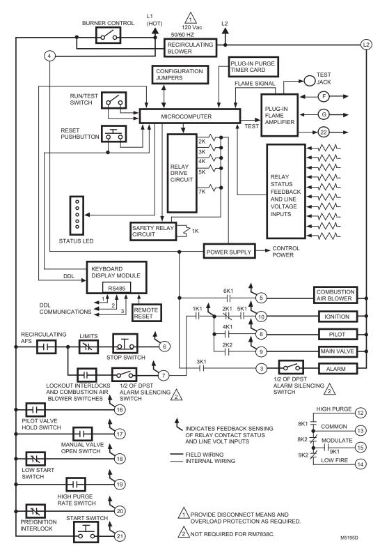
Fig. 2. Internal block diagram of RM7838B,C (see Fig. 3 for RM7838C1020/RM7838C2020); see Fig. 4 and 5 for detailed wiring instructions.
