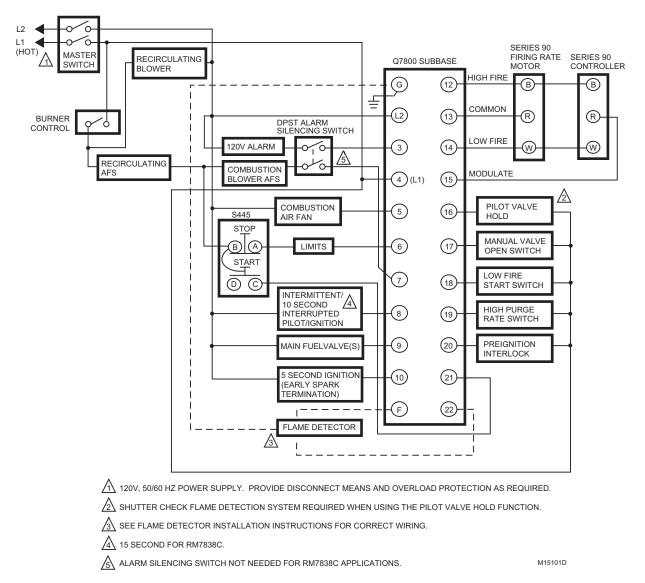
Fig. 4. Wiring subbase for RM7838B,C with S445 Start-Stop Station (not the RM7838C1020/RM7838C2020).
