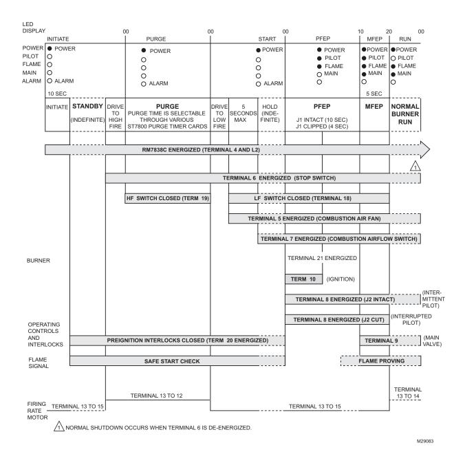
Fig. 9. RM7838C1020/RM7838C2020 Relay Module operation.
