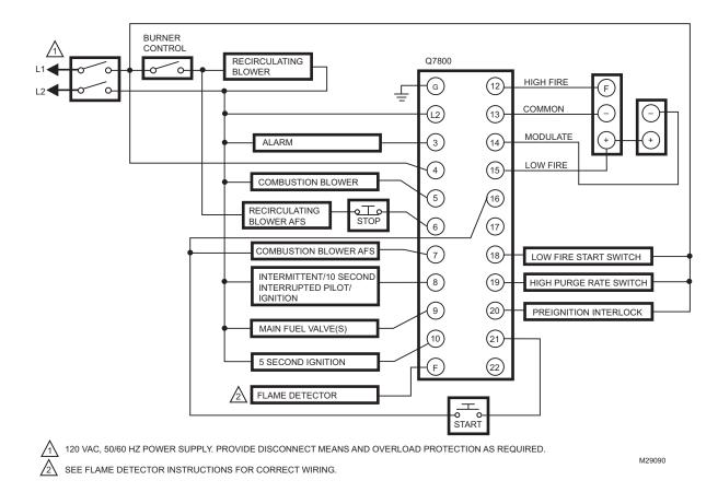
Fig. 6. Wiring subbase for RM7838C1020/RM7838C2020.
