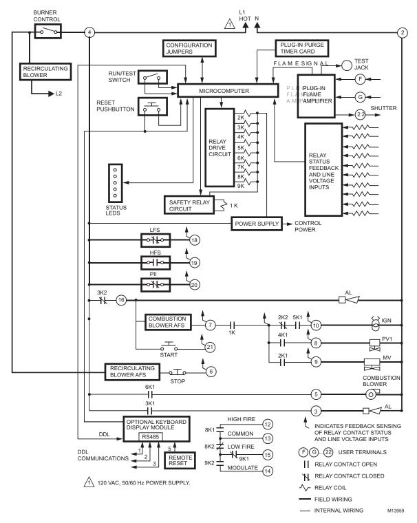
Fig. 3. Internal block diagram of RM7838C1020/RM7838C2020 (see Fig. 6 for detailed wiring instructions).
