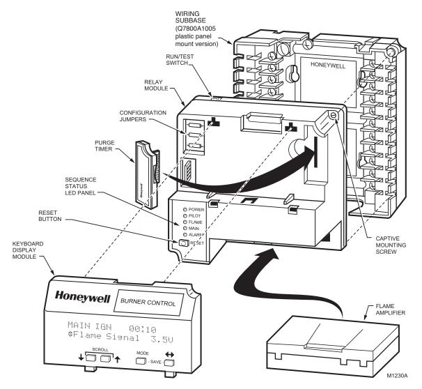
Fig. 7. RM7838B,C Relay Module exploded view.
