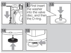
Replace the O-rings on the housing and the valve seat.
