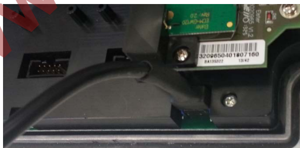
Fig. 10: Local connection using the USB parameterization cable with the EL280 modem parameterizing interface
