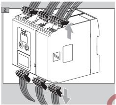
3 Disengage the FCU from the DIN rail.
