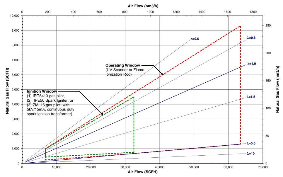
BBG 1006/2006/3006 Operating and Ignition Window Natural Gas 1034 BTU/ft<sup>3</sup> (HHV Standard) / 10.21 kWh/nm<sup>3</sup> (LHV Metric), 0.59 S.G. and Ambient Combustion Air
