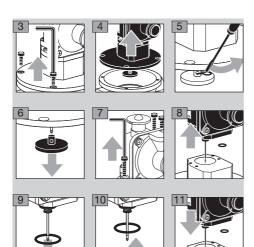
Ensure that the O-ring is fitted in the new measur ing unit, see Figure 11.
