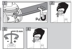
**5** Clearly mark the adjusted value of the outlet pressure p<sub>d</sub> on the type label.
